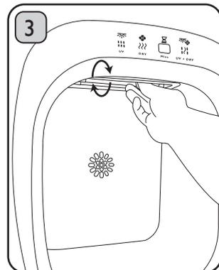
Roll the Bulb away from you within the fitting by 90 degrees until you hear a click. The Bulb is now fitted into position.
