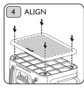
Align the new panel with the screw holes on the body of the toaster.
