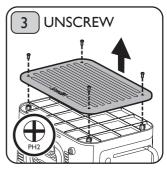
Using a Phillips screw driver (PH2), unscrew and remove panels. **NB. Do not operate the** toaster with the panels removed.
