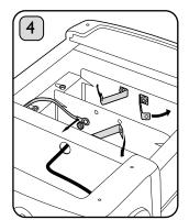
Bend brass links and wires away from the element.
