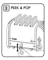
Check the progress of your toast at any time by pushing down on the 'ejector knob'. If you remove your toast before the cycle is complete, cancel timer
