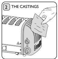
Wipe the aluminium end castings with a damp cloth. Do not use a chemical or abrasive cleaner.
