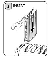
Set 'selector' and starting from the left insert cage into the slots. Push down until clamped tightly shut.
