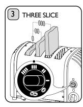
**4 slot model:** Select the three slice indicator. The three slots from the left will toast on both sides.
