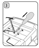
Unscrew brass links and wires.
