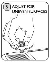
Your toaster is fitted with one adjustable foot which may be raised or lowered to compensate for uneven surfaces. The adjustable foot is located on the base of the toaster and is hexagonal in shape; rotate it to adjust the height.
