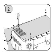
Remove the crumb tray and toaster base plate to access
