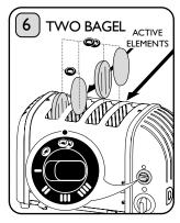
**4 slot models:** Select the two bagel symbol. Only the second and fourth element from the left will heat up.
