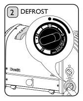
Rotate the 'timer' to the defrost symbol and let the timer wind down to '0'.
