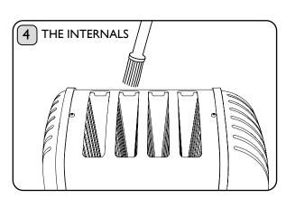
With the toaster unplugged from the power supply use a **SOFT BRUSH** to clean inside your toaster, do not use a sharp or metal utensil! Crumbs should be carefully brushed off the elements using only a soft brush, the toaster can be turned upside down and excess crumbs be shaken out.
