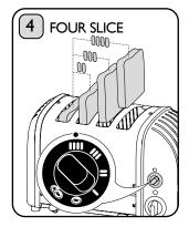
**4 slot model:** Select the four slice indicator. The four slots from the left will heat up on both sides.
