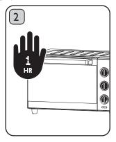
Let the oven cavity, heating elements and protective glass cover cool down for at least an hour after use then remove the wire shelf.
