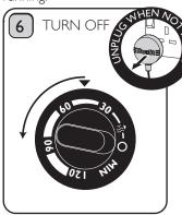
If you need to turn the oven off before the Timer has finished, set the Function Dial to '0' and turn the Timer to '0'. You will hear the bell. **Unplug when not in use Risk of fire**
