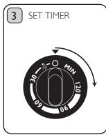
The Timer is the main ON/OFF switch. Turn the dial to the required amount of time. The red light will illuminate when the Timer is running.
