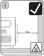
Place the oven on an open, level surface. Ensure there is a 20cm gap between the back of the oven and the wall. Never place below or against a flammable surface. Never block or obstruct the Hot Air Exhaust. Risk of injury.
