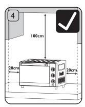
Ensure the oven is positioned at least 100cm clear from any overhanging cupboards and 20cm clear from walls or nearby cupboards on all sides. **Risk of fire.**
