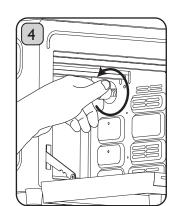
Unscrew anticlockwise and replace the Lightbulb with a new bulb suitable for high temperatures (230°C) having the following specifications: type E14, 240V, 25 watt.
