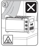
Do not store or use your oven in an appliance garage or under cupboards. Caution: Your oven has a Hot Air Exhaust at the rear. Do not block or obstruct. Risk of fire. Do not touch Hot Air Exhaust. Risk of scalding.
