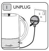
Unplug and empty the kettle. Ensure it has cooled down to room temperature. Risk of scalding and electric shock.
