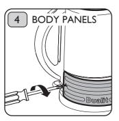
Align the new panel with the screw holes on the body of the kettle and tighten the first screw.
