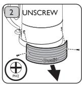
Using a Phillips screw driver (PH2), unscrew and remove the lid and body panels.
