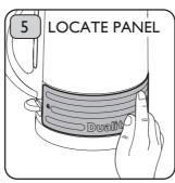
Ensure panel is fully located into recess.
