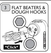
The Flat Beaters and Dough Hooks are marked to indicate which holes they should be inserted into. Always ensure they are in the correct holes and firmly pushed into place, with a click. **Caution - failure** to fit the attachments in the correct hole will cause permanent damage to your Hand Mixer.
