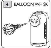
The Balloon Whisk can fit into either hole. Grasp the handle of the Mixer with one hand and the Whisk stem with the other hand. Insert the Whisk with a slight twist and push action until it clicks into place.
