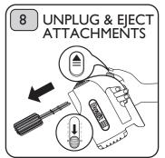
After you have finished mixing, turn the Speed Control to '0' and unplug. Raise the Mixer Head and press down on the Eject Button to eject the Beaters. Note: The Speed Control must be set to '0' to release to Reaters
