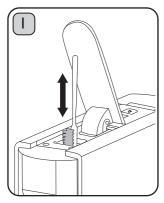
Unplug machine and allow to cool. Use a small brush such as a soft toothbrush to remove any build up of debris on the Filter Plate. A torch is useful to check the plate is completely clean. Once clean, follow the descaling process on page 13 to clean inaccessible parts within the machine. **Caution:** Do not use sharp implements. **Risk of product damage.**
