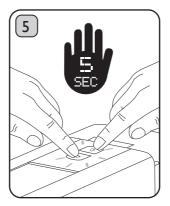
Insert Water Tank, plug in and press either Button to switch on. Press **both** Buttons firmly at the same time and hold for 5 seconds. Both Buttons will then flash quickly. The machine is now ready to descale.
