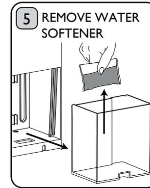
Remove the Water Tank from the back of the appliance, remove the Water Softener Bag and place to one side. Empty the Water Tank.
