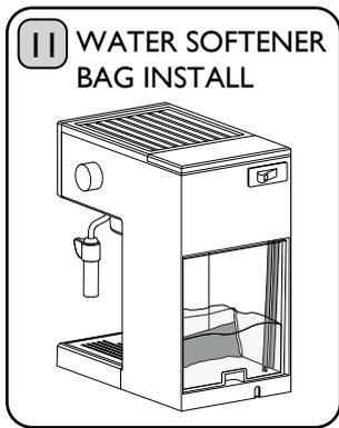
Once the Water Tank has been filled, follow instructions provided with Water Softener Bag to install in the Water Tank. Place Water Tank back into the machine. Ensure that the Water Tank Pipes are positioned into the Water Tank.
