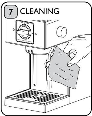
Flush the Steam Wand by dispensing hot water or steam to remove milk residue from inside Steam Wand. Wipe the Steam Wand with a damp cloth. **Product failure due to build-up of milk residue is not covered by your guarantee.**
