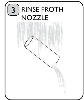
Ensure that the Froth Nozzle is cool before cleaning. Pull the Froth Nozzle off the Steam Wand and wash under running water to remove any milk residue. **Risk of burns.**
