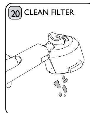
Remove Filter Holder from the Grouphead and knock out the grounds over a bin. Rinse the filter under running water to remove any coffee grounds. Use a pin to unblock if required. **Caution: Filter Holder will be hot. Always hold by the handle, do not touch the metal Filter Basket. Risk of burns and scalding.**
