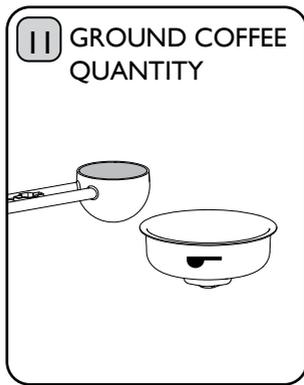
Using the Measuring Spoon, measure out one level Spoon (6-9 grams) per serving into the Cup Filter. Use 2 level Spoons (12-18 grams) if using the 2 Cup Filter. THESE ARE APPROXIMATE, EXACT QUANTITY DEPENDENT ON BEANS AND GRIND SIZE.
