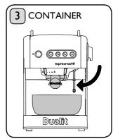
Place a container with a capacity of more than I litre on the Drip Tray underneath the Holder. **Caution: Do not remove the Drip Tray.** Remove Froth Nozzle from the Steam Wand. Direct Steam Wand into container.
