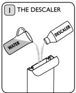
Ensure your descaling product is suitable for coffee machines; follow descaling product instructions carefully. Fill Water Tank with the descaling solution. Descale once a month in hard water areas.
