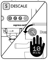
Tum dial fully to the left and empty half of the tank. Then tum dial completely to the right to dispense the remaining water through the steam wand. WARNING: ensure that the switch is set to water, not steam. Wait 10 minutes for descaling to take effect, prior to stage 6.
