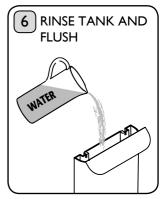
Once machine is descaled, discard descaling solution. Thoroughly rinse Water Tank and repeat steps 2-5. Flush at least two full tanks of fresh water through the machine, Filters and Steam Wand to remove any traces of descaling solution.
