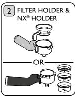
Place the Holder most frequently used into the machine, ensuring it is empty. If both Holders and Filters are used frequently, cycle between them. **Do not soak the holders in descale solution.** Ensure they are rinsed thoroughly after descaling.
