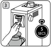
Press & hold the Descale Button for 5 seconds. The Indicator Light will flash red.
