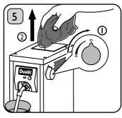
Turn the Steam Valve clockwise fully (1), then remove the plastic bag & tea towel <sup>(2)</sup>.
