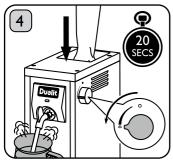
Turn the Steam Valve fully anti-clockwise. Gently apply downward pressure to the plastic bag; until water comes out of the Steam Nozzle. Note this may take up to 20 seconds.
