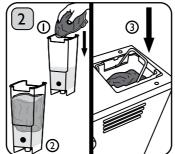
Fill Water Tank halfway (425ml). Place a tea towel in a plastic bag & place it in the Water Tank (1), above the water level to create a tight fit in the Water Tank <sup>(2)</sup>. Place the Water Tank back inside the machine (3).
