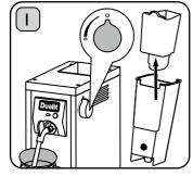
Ensure the Steam Valve is at 0. Turn on by pressing the ON/ OFF Switch. Position the Milk Jug below the Steam Nozzle, remove Water Tank, then the Water Filter Holder & set the Water Filter Holder aside.
