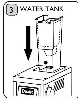
Place the Water Tank into the machine, pressing down firmly. Ensure the Float is facing towards the front. The Water Tank Lid will sit flush with the top surface when the Water Tank is fitted correctly.
