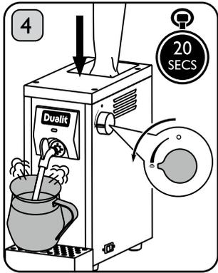
Turn the Steam Valve fully anti-clockwise. Gently apply downward pressure to the plastic bag until water comes out of the Steam Nozzle. Note this may take up to 20 seconds. **Caution: Steam & Hot Water from nozzle, risk of scalding.**
