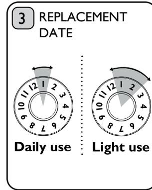
Once Water Filter has been replaced, turn the Water Filter Replacement Indicator to the required month.
