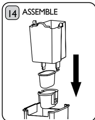
Close Steam Valve. **CAUTION: Keep hands away from the Outlet.** Remove the Water Tank and re-insert the Water Filter Holder and Dualit Water Filter.
