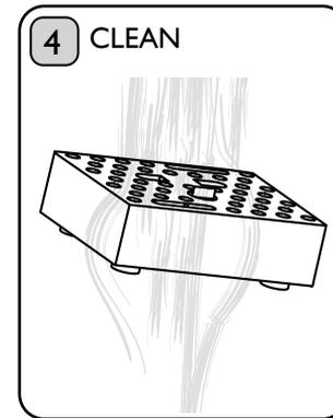
**CAUTION: Allow Drip Tray to cool down before emptying.** Clean Drip Tray with warm soapy water using a non-abrasive pad and dry. Wipe up any Descaler overspill.
