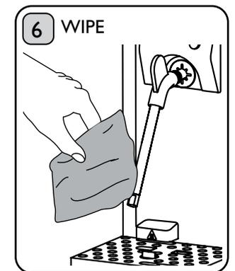
After each frothing, open the Steam Valve to clean. Immediately wipe the Steam Wand with a damp cloth. **Warning: Steam Wand will be hot.** Turn the machine off using the ON/OFF switch and unplug.
