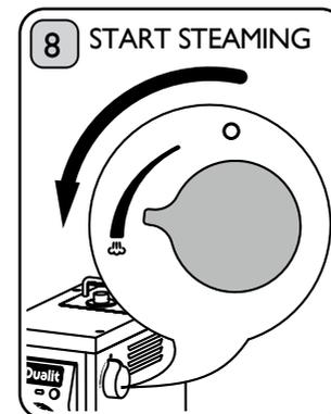
Open Steam Valve; steam will dispense initially, followed by Descaling solution. Dispense all solution. Indicator Light will flash Red and Amber when Water Tank is empty.
