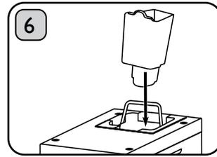
With the Water Tank still inside the machine, place the Water Filter Holder back inside the Water Tank.
