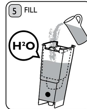
Fill the Water Tank with fresh water until the Dualit Water Filter is submerged. Maximum fill level is the top of the Water Filter Holder. Do not overfill.
