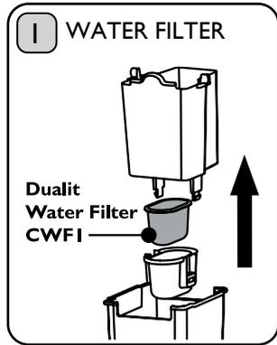
Remove the Water Filter Holder and disassemble. Place 1x Water Filter inside the Filter Basket. Click the Filter Basket back onto the Water Filter Holder and locate in Water Tank.
