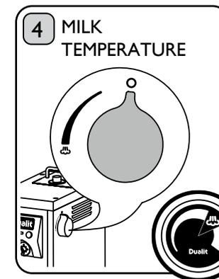
**Warning:** Never lift the Steam Wand Nozzle out of the milk whilst Steam Valve is open. The Steam symbol on the Thermometer indicates recommended milk temperature. When desired milk temperature is reached, close the Steam Valve.
