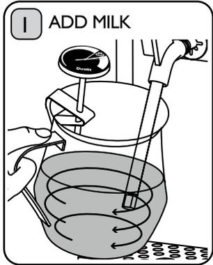
Add milk to the jug. Holding the Jug by the handle, and at a slight angle, place the tip of the Steam Wand Nozzle 1-2 cm below the surface. The wand should be close to the edge of the jug, not in the centre.
