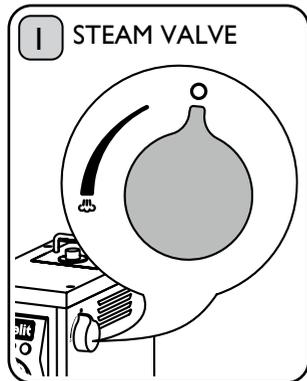
**CAUTION:** Ensure the Drip Tray is located against the front of the machine. Ensure the Steam Valve is in the closed position. **Warning - Risk of Scalding-** Keep hands away from the Outlet at all times.
