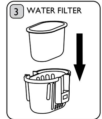
Place one Dualit Water Filter into the Filter Basket, ensuring the rounded end is placed in first. The flat end should sit within the Filter Basket when correctly located.
