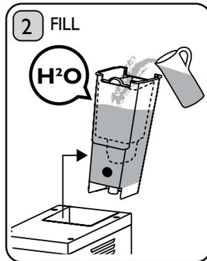
Remove the Water Tank and pour fresh water into the Water Filter Holder. The water will flow through the Filter. Top up as the level drops. Maximum fill level is the top of the Water Filter Holder. Do not overfill.
