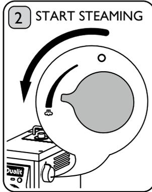
Slowly open the Valve. The steam will flow from the Nozzle and start to rotate the milk like a whirlpool. To speed up the process, gradually open Steam Valve. Take care not to splash the milk.
