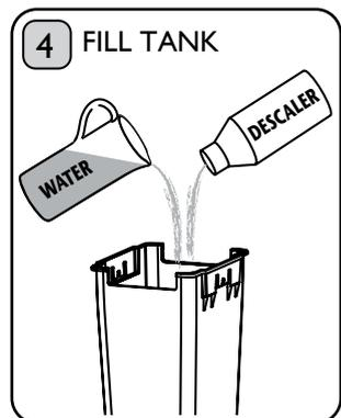
Fill Water Tank with 1 litre of Descaler Solution. **Follow instructions & safety precautions on the Descaler packaging;** Dualit recommends using Kilrock Espresso & Coffee Machine Descaler. If using granular descaler, ensure it is fully dissolved before switching the machine on.
