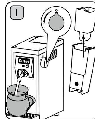
Ensure the Steam Valve is at 0. Turn on by pressing the ON/OFF Switch. Position the Milk Jug below the Steam Nozzle, remove Water Tank, then the Water Filter Holder & set the Water Filter Holder aside.
