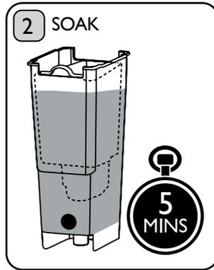
Soak for 5 minutes to activate the Water Filter. Discard the water. The Water Filter only needs to be activated before first use. From then on, you can fill the Water Tank as normal.
