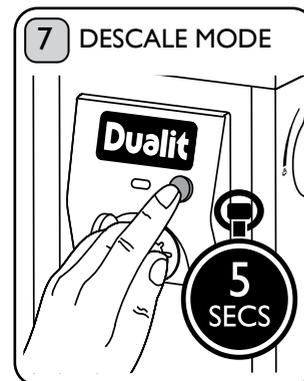
To enter the Descale Mode; Press and hold the Descale Button for **5 seconds**. Once released the Indicator Light will quickly flash red to indicate machine is in Descale Mode.
