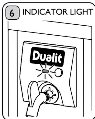
Depending on the machine's status the Indicator Light will be flashing Green, Amber or Red whilst warming up. Once machine is warmed up the Indicator Light will stop flashing and remain on.
