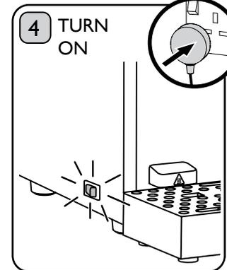
Plug the machine in and turn on. The ON/OFF switch will illuminate Red.
