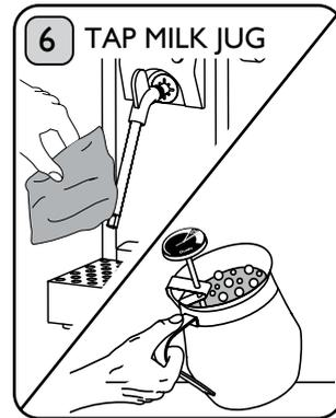
Immediately after frothing, open the Valve and wipe wand to clean. Gently tap Milk Jug against the worktop to collapse any large bubbles. Swirling will mix the milk with the froth. Pour immediately. Turn machine off and unplug.
