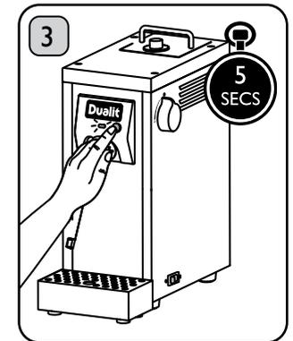
Press & hold the Descale Button for 5 seconds. The Indicator Light will flash red.
