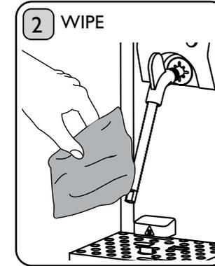
Thoroughly wipe the Steam Wand to clean off any milk residue with a damp cloth. **CAUTION: Steam Wand will be hot.**
