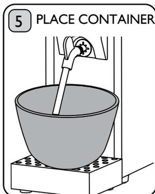
Place Water Tank back into machine. Place a container with a capacity of more than 2 litres on top of the Drip Tray, located under the Steam Wand. Ensure Drip Tray is located against the front surface of the machine.
