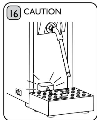
**CAUTION: RISK OF SCALDING.** Keep hands away from the Outlet at all times. Steam/Water will expel from Outlet when Steam Valve has been closed. This is normal operation.
