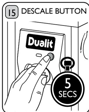
Press and hold the Descale button for **5 seconds** to exit. Indicator Light will flash Green whilst warming up. Indicator Light will stop flashing and remain on when ready.
