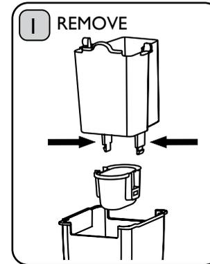
Remove Water Tank Lid. Remove the Water Filter Holder from the Water Tank. Remove the Filter Basket by pinching both tabs on the Water Filter Holder and pull the Filter Basket off.
