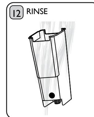
Remove Water Tank and rinse with fresh water. Fill Water Tank with fresh water and place back in the Machine.
