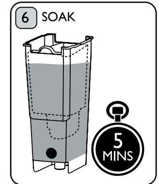
Soak for 5 minutes to activate the Dualit Water Filter. Discard the water. The Dualit Water Filter only needs to be activated before first use. From then on, you can fill Water Tank as normal.
