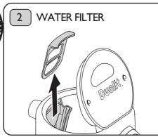
Unplug and let the kettle cool. Open the lid. Hold the top of the filter, pull up and out of the kettle. Rinse under a tap while carefully brushing it with a soft brush. Rinse the kettle out with fresh water. To replace, align the filter with the grooves in the filter holder, insert and push back into place. **DO NOT OPERATE KETTLE UNLESS THE WATER FILTER** IS CORRECTLY IN POSITION.
