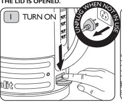
Plug the kettle into the power socket. Press the 'On/Off' switch down. The power neon will illuminate and the kettle will start to heat up. If the kettle is accidentally switched on with no water inside, the boil-dry device will switch off the heating element to prevent damage to the kettle.
