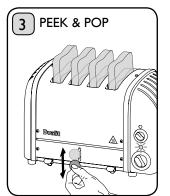
Check the progress of your toast at any time by pushing down on the 'ejector knob'. If you remove your toast before the cycle is complete, cancel timer and unplug.
