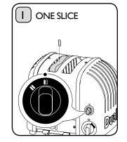
**2, 3 & 4 slot models:** Select the one slice indicator on the 'selector switch'. The left hand slot will heat up on both sides.
