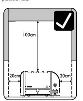
Ensure the Toaster is positioned at least 20cm CLEAR FROM ANY OVERHANGING CUPBOARDS.
