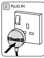
The toaster will only engage when the power is switched on. Plug the toaster into the wall power socket and turn power on at socket. 2 SET CIRCLE INDICATOR
