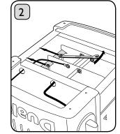
Unplug and place toaster on a soft cloth. Remove crumb tray and unscrew feet to remove the base plate. Loosen locking nuts on retaining plate using a 6.5mm spanner and slide back. Ensure that the retaining plate is correctly in position when reassembling.
