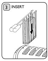
Set 'selector' and starting from the left insert cage into the slots. Push down until clamped tightly shut.
