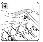
The fuse is reset by depressing the small white button on its face.
