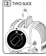
**2, 3, 4 & 6 slot models:** Select the two slice indicator. The two slots from the left will toast on both sides.
