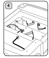
Bend brass links and wires away from the element.
