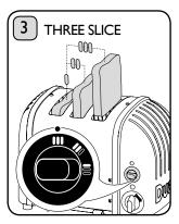
**3 slot model:** Select the three slice indicator. The three slots from the left will toast on both sides.
