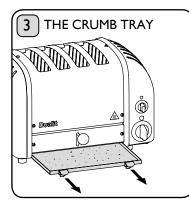
Crumbs will accumulate in the crumb tray and could catch fire if the tray is not emptied frequently. Pull out the crumb tray and wipe clean using a damp cloth. **CRUMB TRAY MUST BE IN PLACE DURING TOASTING.**
