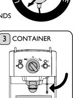
Place a container with a capacity of more than I litre on the Drip Tray underneath the Holder. **Caution: Do not remove the Drip Tray.** Remove Froth Nozzle from the Steam Wand. Direct Steam Wand into container.
