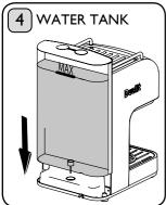
Insert Water Tank. Plug machine in and turn on; wait until machine has reached operating temperature. **Caution: Keep hands away from Steam Wand at all times.**
