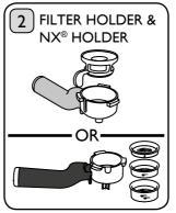
Place the Holder most frequently used into the machine, ensuring it is empty. If both Holders and Filters are used frequently, cycle between them. **Do not soak the holders in descale solution.** Ensure they are rinsed thoroughly after descaling.
