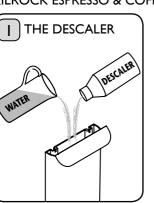
Ensure your descaling product is suitable for coffee machines; **follow descaling product instructions carefully.** Fill Water Tank with the descaling solution. **Descale once a month in hard water areas.**
