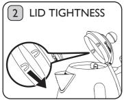
Tip: If the Lid is too tight, try pushing in the pips on the inside of the Lid with a spoon handle. Pushing the Lid Pips back out will give a tighter fit. **WARNING:** IF THE LID IS TOO LOOSE, **RISK OF SCALDING.**
