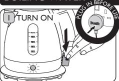
Plug the kettle into the power socket. Press the 'On/Off' switch down. The power neon will illuminate and the kettle will start to heat up. If the kettle is accidentally switched on with no water inside, the boil-dry device will switch off the heating element to prevent damage to the kettle.
