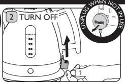
The kettle will automatically turn off after the water has boiled and the neon light will go out. To turn off before the water has boiled lift up the On/Off Switch. **DO NOT LEAVE THE** APPLIANCE UNATTENDED DURING **USE. UNPLUG AFTER EACH USE. RISK OF FIRE IF AN UNATTENDED APPLIANCE IS LEFT OPERATING OR** PLUGGED IN.
