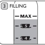
Fill the kettle through the Lid opening. Use at least one cup of water (250ml). The water level must stay below the 'Max' Mark Indicator. Save energy, only boil what you require. Keep kettle upright and level at all times when filling (maximum 15° incline). Do not tilt kettle backwards. **DO NOT OVERFILL** OR FILL THROUGH THE
