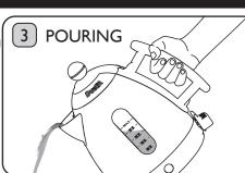
Remove kettle from the Power Base. When filling or carrying the kettle, do not tilt it backwards, as this may allow water to pass through the Steam Tube onto the control area. Should this happen, the kettle must be allowed to dry before re-using. To avoid the risk of splashing, once the kettle has boiled wait 10 seconds then pour slowly. Do not over-tilt the kettle.
