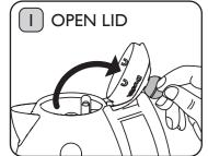
Ensure the kettle is unplugged. Remove the kettle from the Power Base. Pull the Knob up and towards the handle to open the lid. The Lid is hinged for easy opening and closing.
