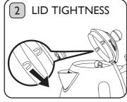
Tip: If the Lid is too tight, try pushing in the pips on the inside of the Lid with a spoon handle. Pushing the Lid Pips back out will give a tighter fit. **WARNING:** IF THE LID IS TOO LOOSE,
