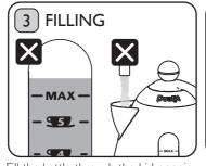
Fill the kettle through the Lid opening. Use at least one cup of water (250ml). The water level must stay below the 'Max' Mark Indicator. Save energy, only boil what you require. Keep kettle upright and level at all times when filling (maximum 15° incline). Do not tilt kettle backwards.
