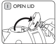
Ensure the kettle is unplugged. Remove the kettle from the Power Base. Pull the Knob up and towards the handle to open the lid. The Lid is hinged for easy opening and closing.
