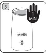
NOTE: If you are using the the Milk Frother for multiple cycles consecutively, you will need to allow time for the Jug to cool. After 2 cycles fill the Jug with cold water and stand for 1 minute before discarding. Repeat after each additional cycle.
