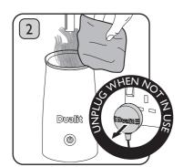
WARNING: Clean immediately after each use. Unplug, remove Jug from Power Base and remove the Whisk and Attachments. Clean inside of Jug, Whisk and Attachments with warm, soapy water and a non-abrasive cloth. Rinse with cold water. Wipe exterior with a damp, non-abrasive cloth. Never immerse the Jug or Power Base in water. Risk of electric shock, fire and product damage.
