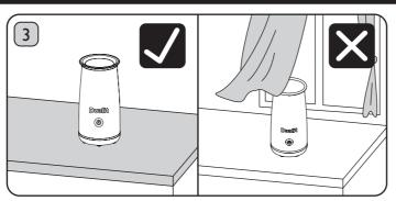
The surface must be flat in order to keep the machine level and stable. **Risk of injury.** Position in a safe space away from:
