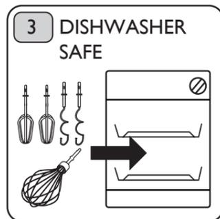
The Beaters, Dough Hooks and Balloon Whisk are all dishwasher safe. Use a wash cycle below 40°C. Remove prior to drying cycle. **The Main Body is not dishwasher safe.**
