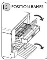
Position the Bread and Toast Ramps as shown above. Note: Once the Bread Ramp has been positioned, it cannot be moved. Dualit recommend having a basket underneath the Toast Ramp to catch toasted items.
