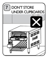
Ensure your Conveyor Toaster is not stored in an appliance garage or underneath cupboards. Overheating may occur if the appliance is not correctly positioned. **Risk of fire.**
