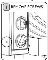
Remove the two screws seen on the left and right-hand sides of the controls. Align the Anti-Tamper Guard with the screw holes.
