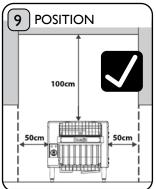
Place the Conveyor Toaster on an open level surface. Ensure that it is positioned 100cm away from any overhanging cupboards or ceilings.
