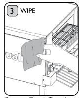
Remove Crumb Tray, tip out all of the crumbs, then clean with a damp cloth and replace. Ensure the area around the Conveyor Toaster is clean and crumb free. Clean the fan air intake with a damp, non-abrasive cloth.
