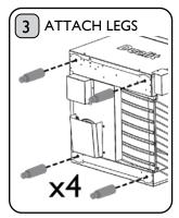
Carefully place your Conveyor Toaster on its side. Thread all 4 legs into the holes shown and tighten using a 21mm spanner. Pick up and place the Conveyor Toaster on its feet. **Caution: do not operate**
