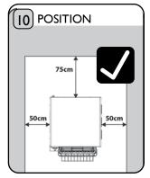
Ensure the Conveyor Toaster is positioned at least 50cm clear from walls. For best results use away from drafts. Warning do not use near water sources.
