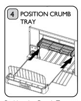
Position the Crumb Tray into the mounting rails beneath the Conveyor Belt. Caution: Failure to do so could cause the appliance to overheat.
