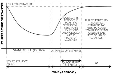
Your toaster is fitted with a temperature limiting thermostat. During periods of inactivity, longer than 5 minutes, the elements will turn off (indicated by the red power indicator going off). Only introduce bread to the conveyor when the red light is on and the elements are glowing cherry red.
