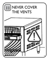
Never cover the vents on the sides of the Conveyor Toaster. This will prevent necessary air flow and could cause a fire.
