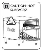
Caution: The surfaces of the Conveyor Toaster will get extremely hot during operation. Ensure to touch only the dials when in use, as risk of scalding. Do not place items on top of the Conveyor Toaster, in particular plastic such as bread bags that could melt.
