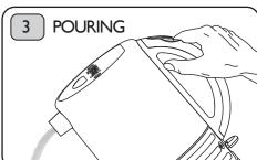
Remove kettle from the power base. When filling or carrying the kettle, do not tilt it backwards, as this may allow water to pass through the steam tube onto the control area. Should this happen, the kettle must be allowed to dry before re-using. To avoid the risk of splashing, once the kettle has boiled wait 10 seconds then pour slowly. Do not over-tilt the kettle.
