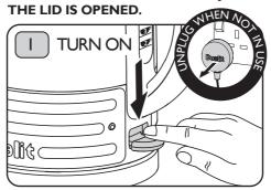
Place the kettle on the Power Base. Plug the kettle into a power socket. Press the On/Off Switch down. The Power Neon will illuminate and the kettle will start to heat up. If the kettle is accidentally switched on with no water inside, the boil-dry device will switch off the heating element to prevent damage to the kettle.
