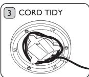
Use the shortest cord possible. Wrap excess cord around the Cord Tidy under the Power Base.
