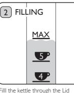
Fill the kettle through the Lid opening. Use at least one cup of water (250ml). The water level must stay below the Max Mark Indicator. Save energy by only heating what you require. Keep kettle upright and level at all times when filling. Do not tilt kettle backwards. **DO NOT OVERFILL OR FILL THROUGH THE SPOUT.**
